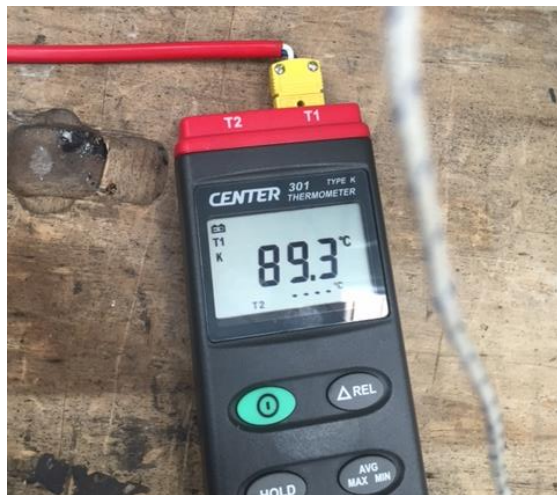
Figure 10: 89.3 °C, temperature recorded at flue gas exit point
