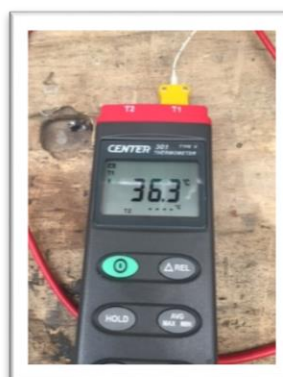
Figure 5: Temperature between outer flue and penetration seal 36.3 °C
