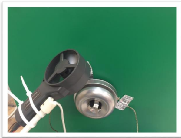
Figure 14: Anemometer placed in the pathway of the flue gas
