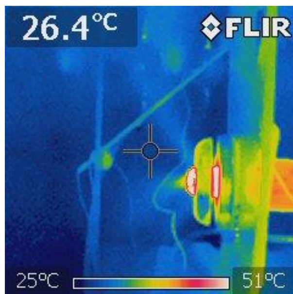
Figure 20: Showing the flue gas plume exiting the flue termination
