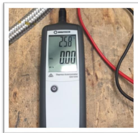
Figure 17: Results from Anemometer 2 and no air speed
