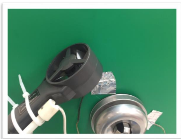
Figure 16: Position of Anemometer close to the Trespa cladding
