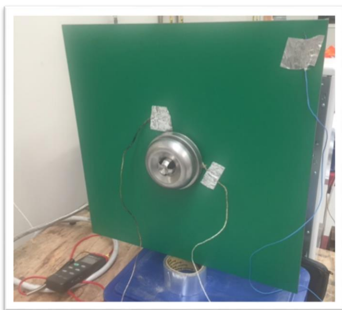
Figure 13: Test setup for the Trespa cladding material
