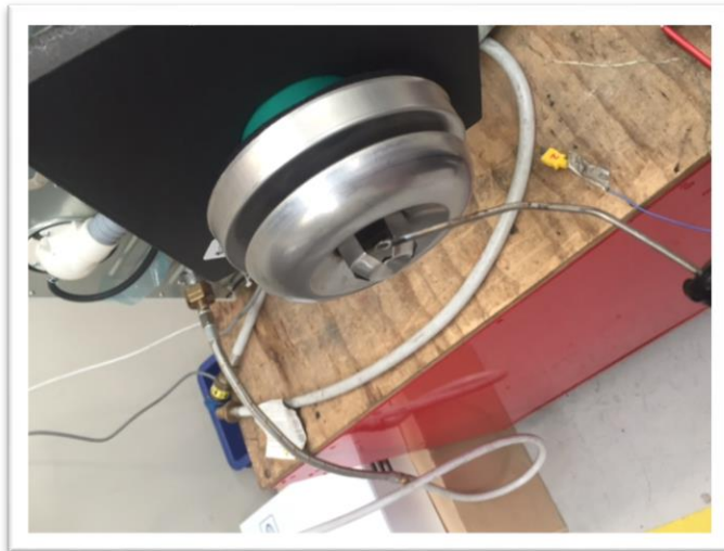
Figure 9: Temperature measurement with hand held thermocouple at flue gas exit point
