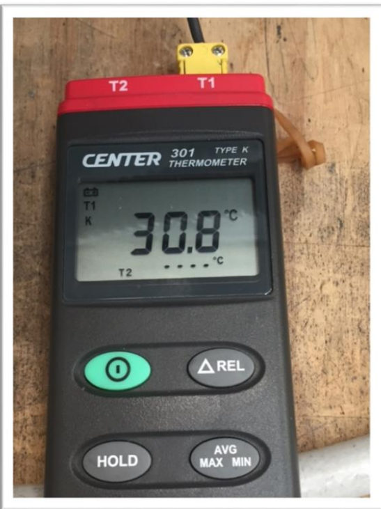
Figure 8: 30.8 °C , temperature recorded at the mushroom flue
