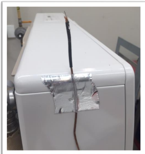
Figure 2: Ambient air temperature thermocouple position
