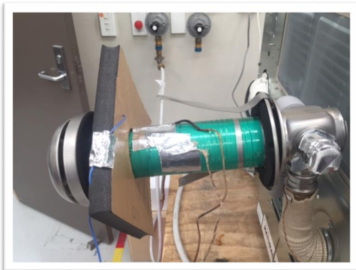
Figure 1: General arrangement of thermocouples on flue and Vanluk MG-100-18-16 penetration seal
