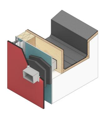
Pipe / Penetration Cavity Flashing System
